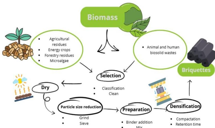
Figure 1. Briquetting process for biomass residues.
