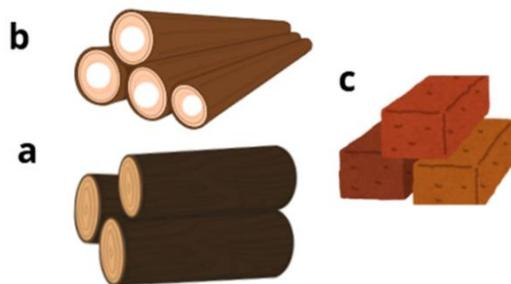
**Figure 3.** Briquette shapes. a) cylindrical briquette; b) cylindrical briquette with a central hole; c) box.
