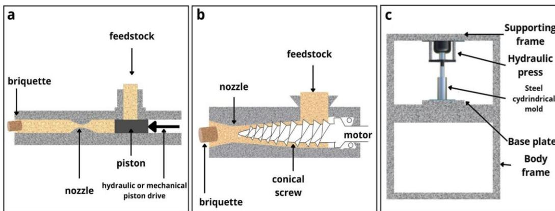
Figure 4. Equipment to produce briquettes. a) Mechanical piston press; b) screw extruder; c) hydraulic press.
