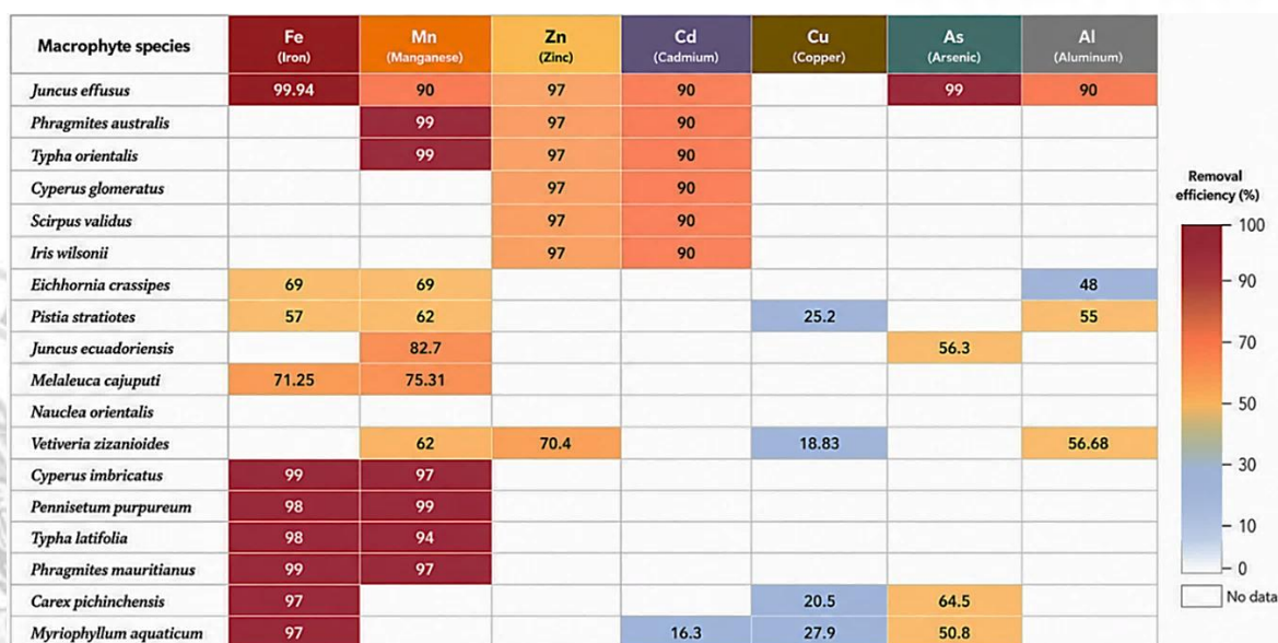
Figure 2. Comparative metal removal efficiency of macrophytes used in AMD treatment. Color intensity represents the removal percentage reported in the reviewed studies. ND: no reported data.
