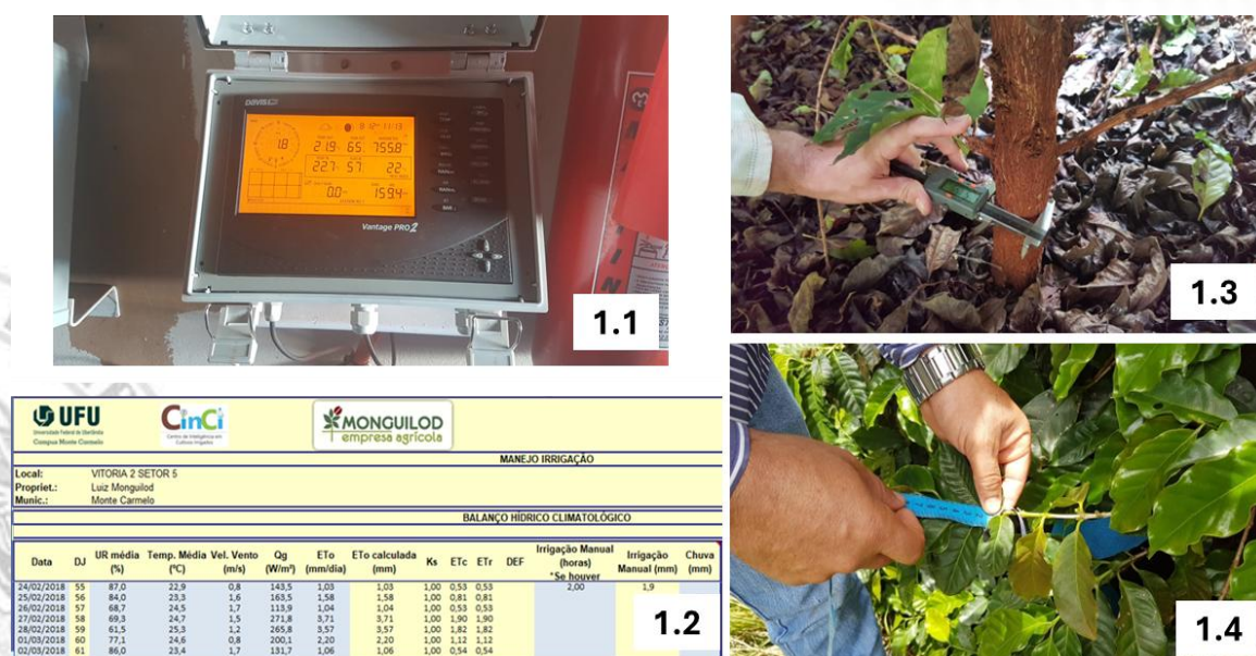
Figure 1. Davis Vantage Pro2 meteorological station panel (1.1), climatic management monitoring spreadsheet in Excel (1.2), coffee tree stem diameter measurement with digital caliper (1.3), and plagiotropic branch length measurement with precision measuring tape (1.4).
