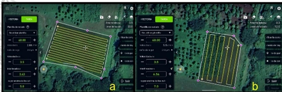
Figure 3. For flight programming, the drone was calibrated and configured to execute the designated treatments. Treatment 1 utilized a flight altitude of 5 m (a), while Treatment 2 employed 7 m (b). Both treatments maintained a constant flight speed of 3.5 m/s, an average droplet size of 310 \mu\text{m} , a double-layer spray pattern and a spray volume of 40 L/ha.
