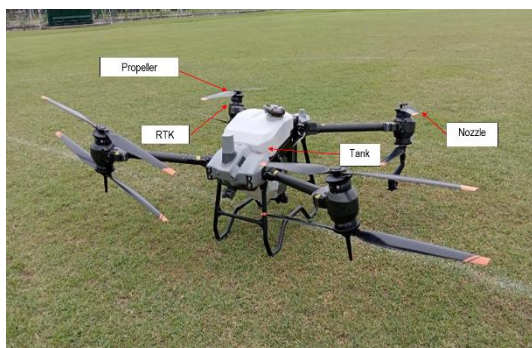
Figure 2. DJI Agras T40 Unmanned Aerial Spraying System (UASS) illustrating the rotary atomization spray mechanism.
