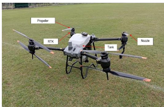
Figure 2. DJI Agras T40 Unmanned Aerial Spraying System (UASS) illustrating the rotary atomization spray mechanism.
