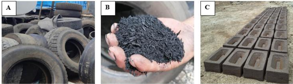
Figure 1. Production of eco-friendly clay bricks: A) Collection of ELTs, B) Shredded recycled rubber from ELTs, C) Clay bricks with incorporated rubber.
